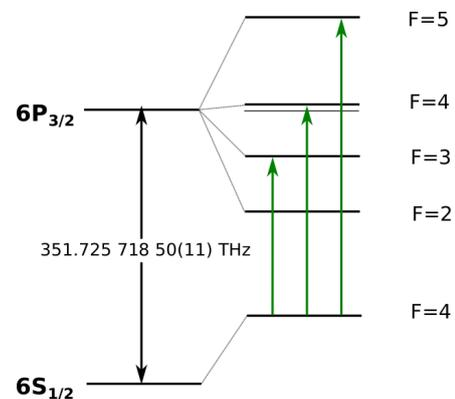
**Fig. 6** Fine and hyperfine structure for the D2 transition for Cesium. In green, the achievable transitions for our laser. Data taken from [4].
