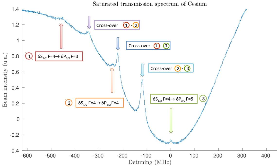
**Fig. 8** Experimental sub-Doppler transmission spectrum of Cesium. Six peaks are observed and correspond to the three available transitions plus the three cross-overs. The x-axis calibration is calculated by using the known frequencies of peaks 1 and 3. Then, we have checked the positions of the other peaks.
