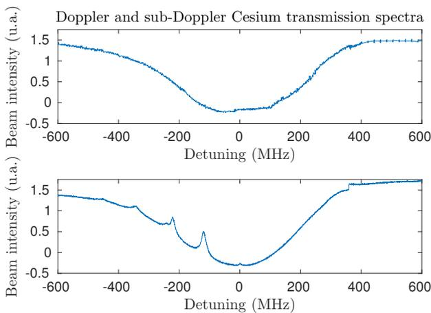
**Fig. 7** Top: Doppler transmission spectrum of Cesium. The gap is due to the D2 transition which is Doppler broadened. Bottom: Sub-Doppler transmission spectrum. The main gap is due to the Doppler broadening of the D2 fine transition and the small peaks represent the hyperfine D2 transition. That illustrates the resolution improvement.
